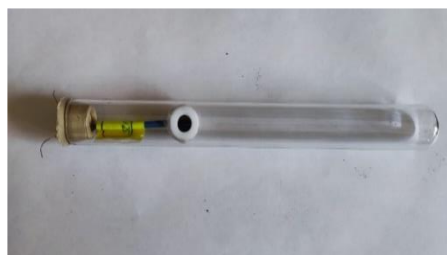
Fig. 3. Sensor in an airtight test tube.
