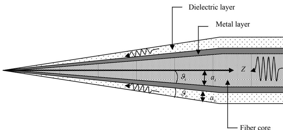
Fig. 1. Longitudinal section of fiber, covered with metal and dielectric layers.
