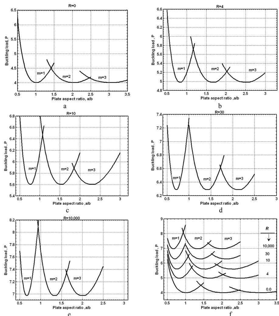
Fig. 2. Non-dimensional buckling loads,  $\bar{P} = Pb^2 / \pi^2 D$ , versus plate aspect ratio  $a/b$ :
