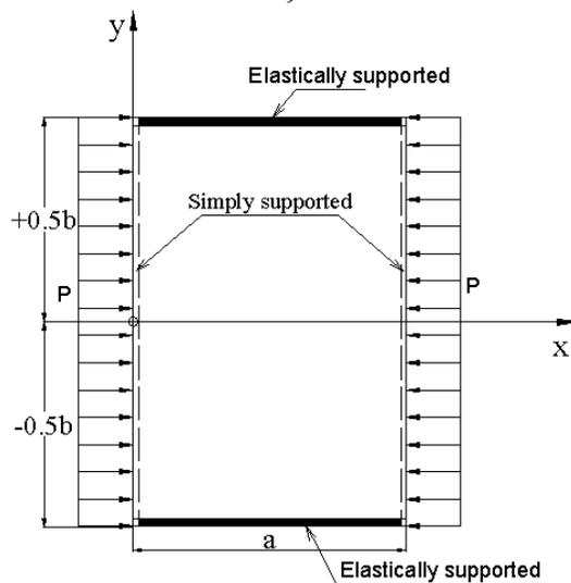
Fig. 1. Uniformly compressed rectangular plate simply supported along the edges  $x=0$  and  $x=a$ , and elastically supported against rotation along the other edges (SSEE plate).
